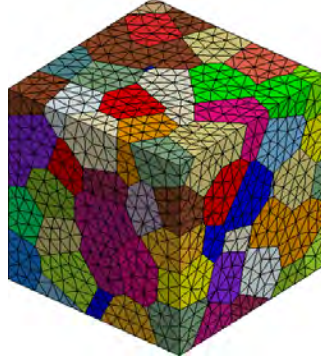
Fig. 3. Aggregate representing a former austenitic phase by 120 Voronoi cells and free mesh. Each color corresponds to one crystallographic orientation
