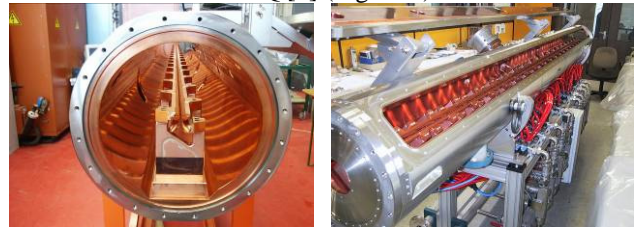
Figure 2: Left: SARAF CW RFQ - 3 MeV 4mA D + , 175MHz; right: indust. 4-rod CW RFQ 176 MHz/220kW.
