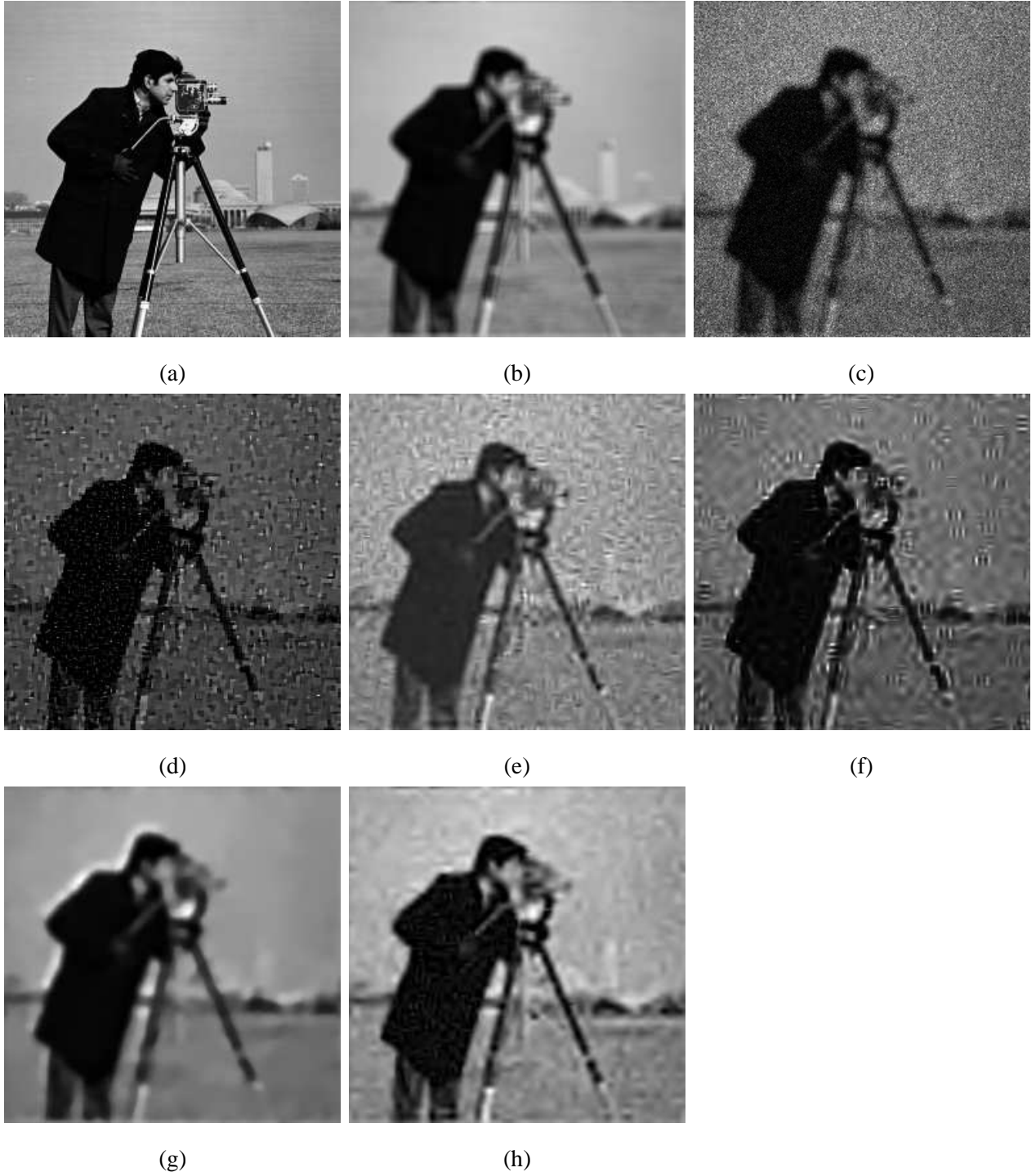
Figure 4. Deconvolution of the cameraman ( \text{Intensity} \leq 30 ). (a) Original, (b) Blurred, (c) Blurred&noisy, (d) RL-TV [7], (e) NaiveGauss [12], (f) RL-MRS [3], (g) FTITPR [55], (h) Our Algorithm.
