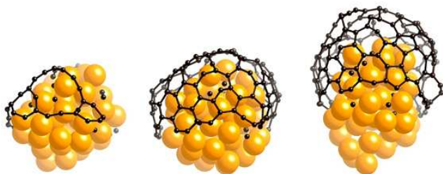
FIG. 12: Successive stages of the nucleation of a C cap on a 55 atom cluster of nickel for a chemical potential equal to 5.25 eV/atom.
