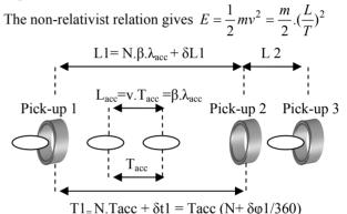
The third pick-up is used to determine the number N of bunches between pick-up 1 and pick-up 2.
