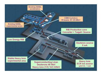
The SPIRAL 2 facility is based on a high-power, superconducting driver LINAC, which will deliver a high-intensity, 40 MeV deuteron beam as well as a variety of heavy-ion beams with mass-to-charge ratio equal to 3 and energy up to 14.5 MeV/u. The driver accelerator will send stable beams in a new experimental area and in a cave for the production of Radioactive Ion Beam (RIB). The commissioning of the driver should start in 2011 at GANIL.
