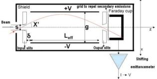
With an energy q.U, an ion (charge q) enters with an angle x', is deviated by a voltage V and goes through output slits. The equation of V is given by:  $V = 2 U x' (\alpha (l \circ f))$
