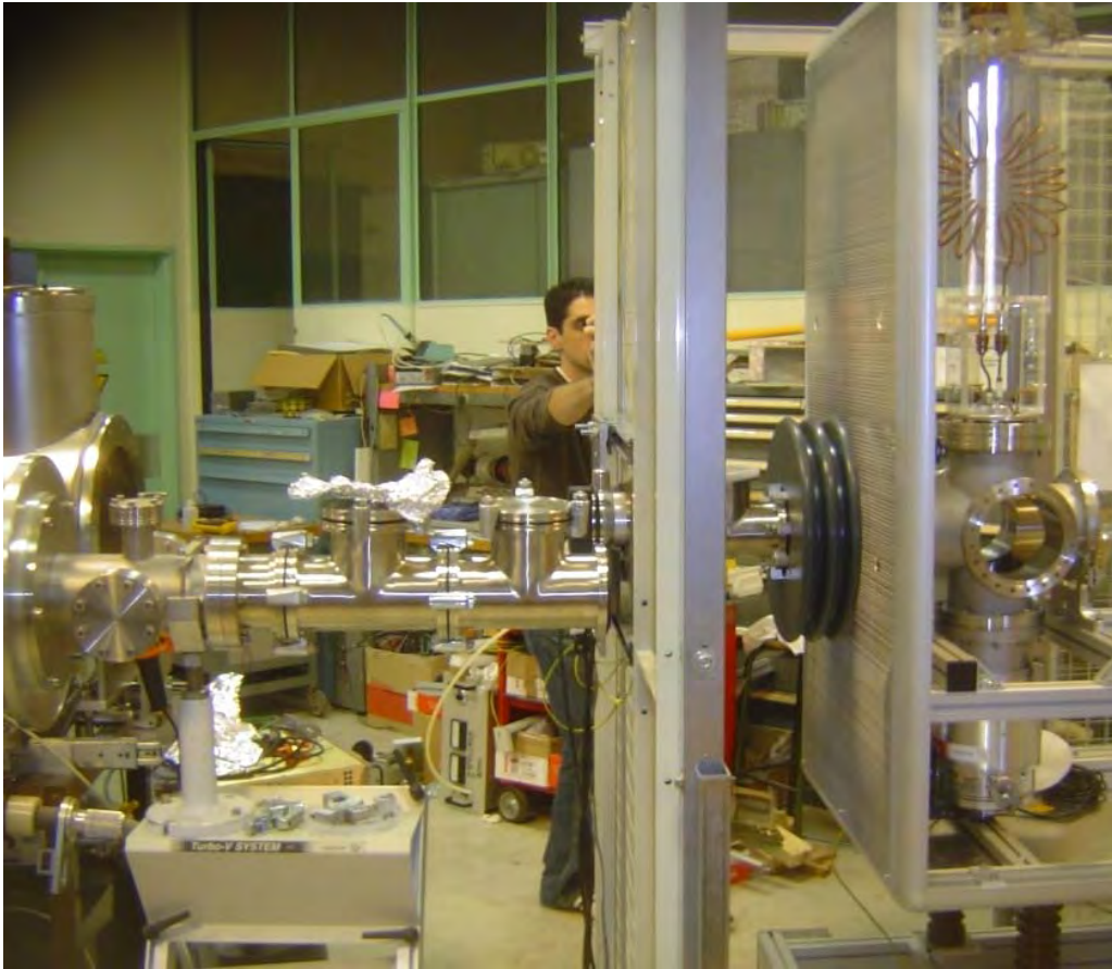
Fig. 6: Photograph of the high-voltage cage (right) that houses the high-current cooler assembly. Also visible (left) is the connecting beam line to the SIDONIE mass-separator at CSNSM in Orsay.
