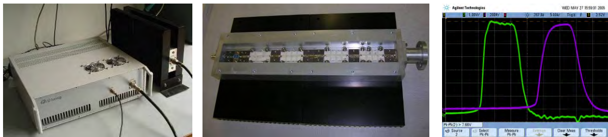
Fig. 13: (Left) pulser and matching load; (centre) resistances inside the load; (right) pulser and load signals.
