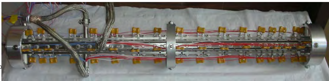
Figure 7: Photograph of the full-length high-current cooler assembly, with connections.
