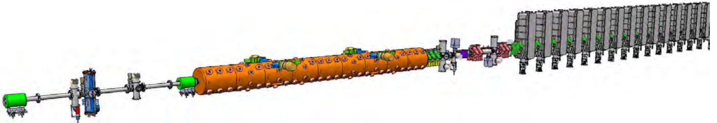
Fig. 2: Low-energy beam line, with pre-buncher and solenoids, RFQ, MEBT, and the first part of the SC linac.
