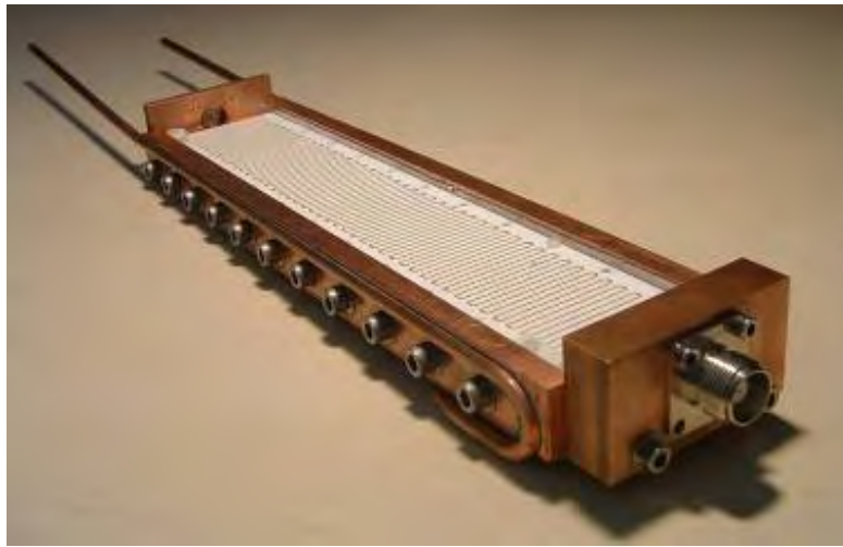
Fig. 15: The ceramic plate with meander-line electrode assembled on the water-cooled support.
