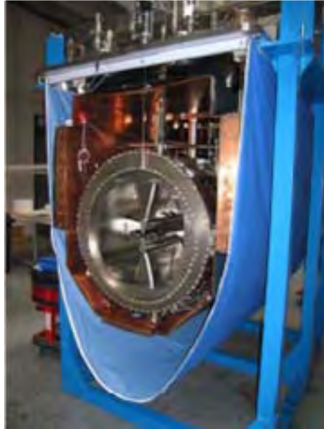
Fig. 8: The PIAVE SC-RFQ resonators in their cryostat.
