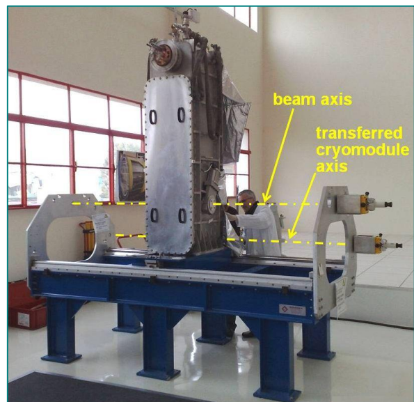
Figure 11: Cryomodule A on the bench for axis transfer operation
