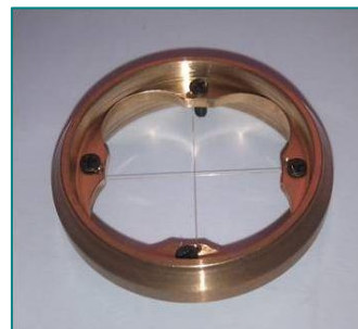
Figure 15: Target comprising crossed gold tungsten threads
