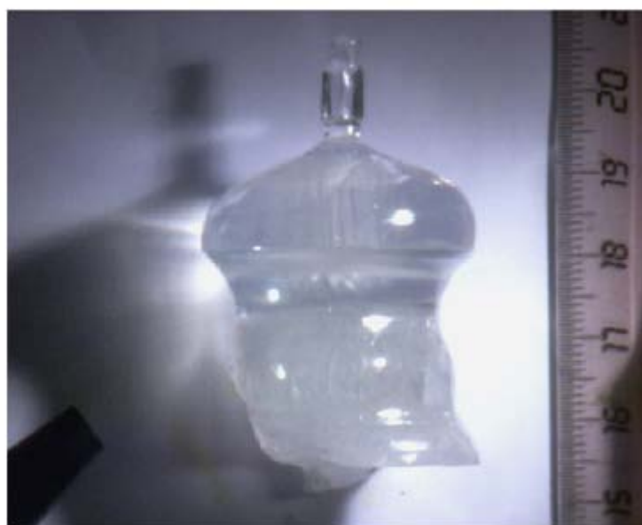
Fig. 2. Photography of an as-grown LGB single crystal.
