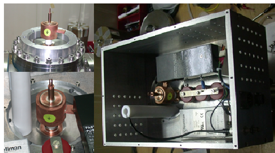
Figure 6: The HV module connected with feed-through.
