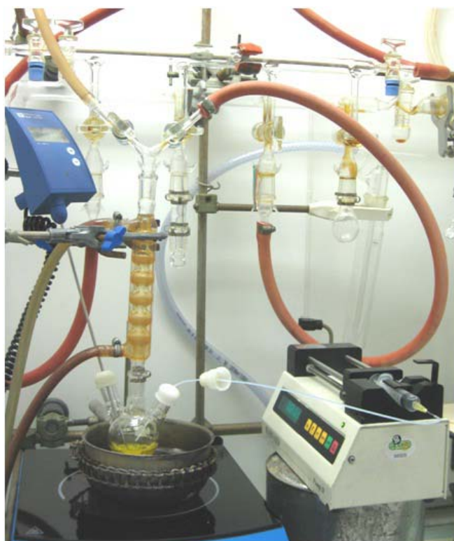
Figure A1.3: Photo of experimental setup for synthesis of \text{In(Zn)P/ZnS} core/shell NCs using \text{P(TMS)}_3
