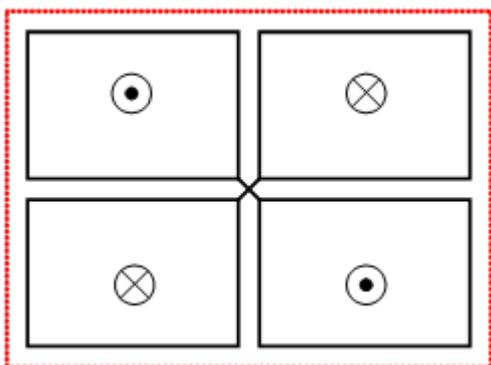
Figure I-31 – L'antenne double-Huit
