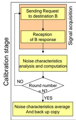
Figure IV-45 – Phase de calibration
