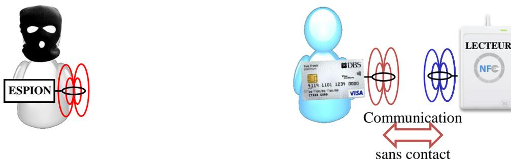
Figure I-7 – Attaque eavesdropping
