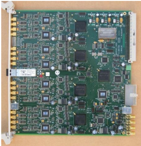
Figure 10: the 16-channel WaveCatcher board
