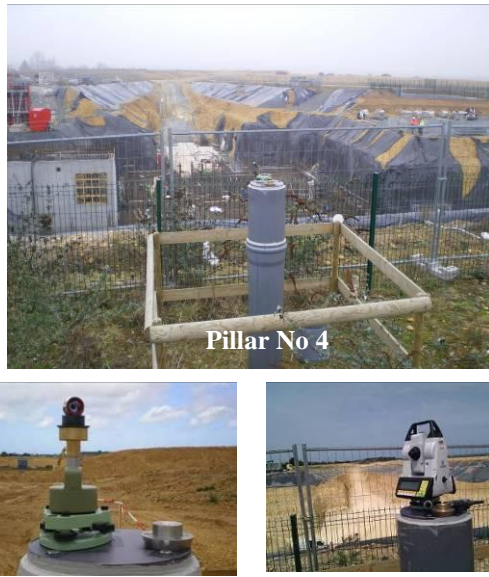
Figure 5: View of the upper section of a geodesic pillar
