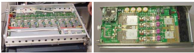
Figure 4: Example of 1 and 2 kW standard FM units. (Courtesy of R&S and ECRESO)
