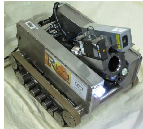
Fig. 9: RICA III robot (gamma camera, dose rate measurement, gamma spectrometry, telemetry)
