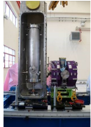
Figure 10: left - Laminar air flow in-between cryomodules in the linac tunnel, right – test of the assembly between a warm section and a CMA in Saclay.
