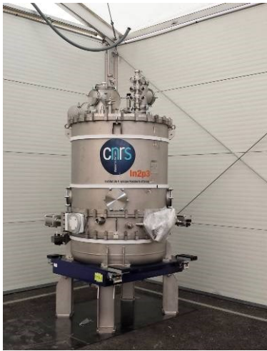
Figure 5: The first cryomodule in GANIL, ready for installation in the linac tunnel.
