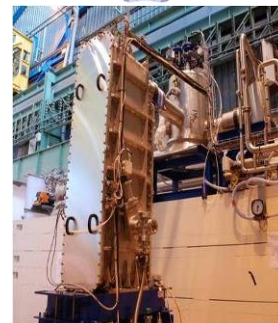
Figure 3: The SPIRAL2 superconducting cryomodules (left: \beta_0=0.07 – 1 cavity, right: \beta_0=0.12 – 2 cavities).
