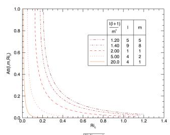
**Fig. 1.** Attenuation rate Att =  $e^{-\pi \sqrt{\frac{l(l+1)}{m^2} R_{i_c} - \frac{1}{4}}}$  of the wave passing through a critical layer as a function of the Richardson number. We observe that Att increases with  $\frac{l(l+1)}{m^2}$ .
