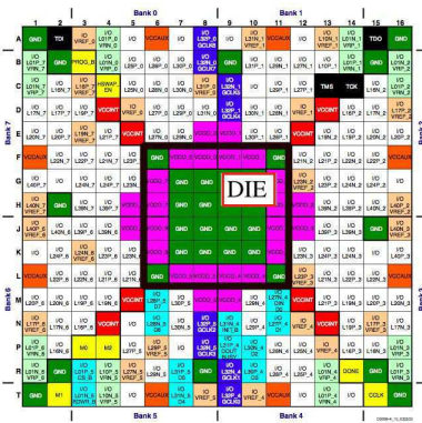
Fig. 2. The FPGA package footprint [4]
