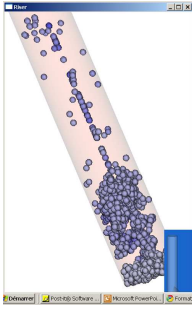
Figure 4: Another view during runtime. The spheres represent the solid macro-particles. We can see an emerging privileged solid path near the axis of the riser cylinder. At the bottom of the cylinder, one can see a strong concentration of solid catalyst particles that form the fluidized bed.
