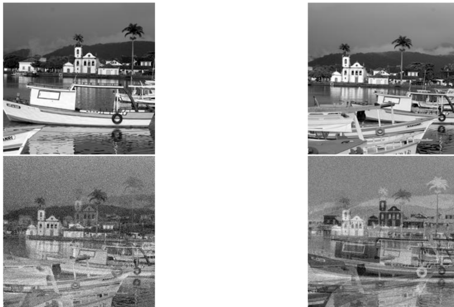
Figure 1. Top : the 256 \times 256 source images. Bottom : two different mixtures. Gaussian noise is added such that the SNR is equal to 10dB.
