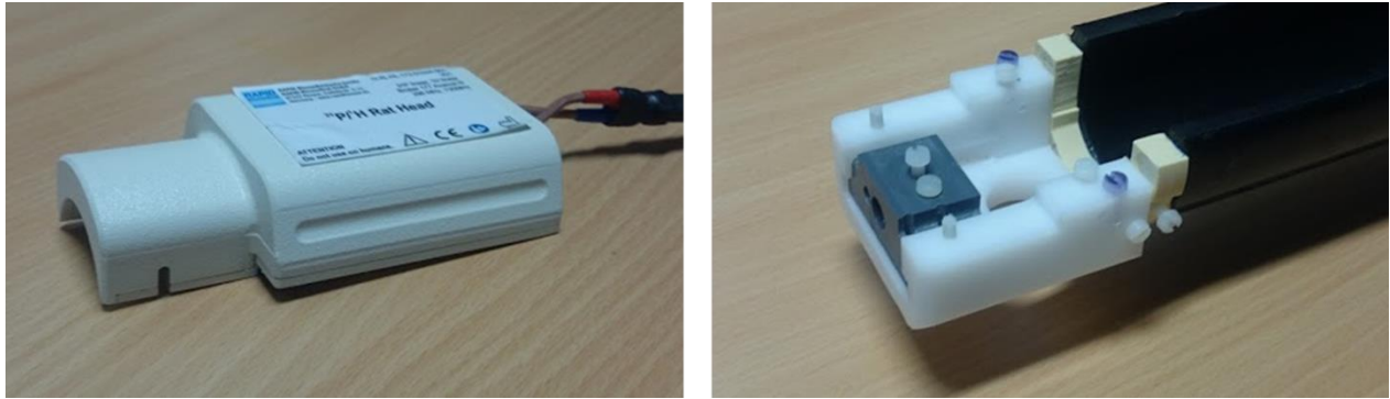
Figure 4.1. Dual ^1\text{H}/^{31}\text{P} coil and a dedicated home-made holder used for ^{31}\text{P} MRS experiments.
