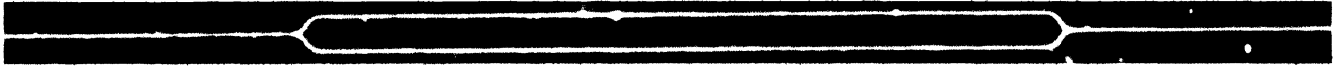
Figure 7: Optical photograph of a Mach-Zehnder interferometer structure etched in a 2 \mu\text{m} thick PZT (36/64) film on glass substrate.
