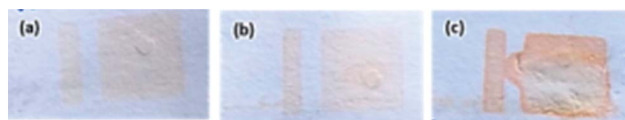
Fig. 11 Photographs of printed solid forms on cellulose substrates after irradiation and rising steps: (a) 1-pass printing, (b) 3-pass printing and (c) 6-pass printing.
