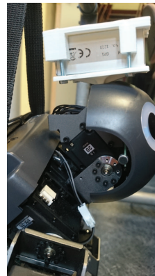
Fig. 2: GR1 detector attached to H@RI's head
