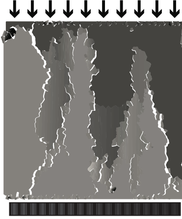
Figure 17: Pure compression test simulation with the virtual testing machine.
