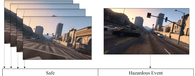
Fig. 1: Demonstration of our hazardous event labelling technique, tested on a pre-labelled simulation benchmark, GTACrash. The triggering event was detected using vehicle kinematics and calculated safe distances.
