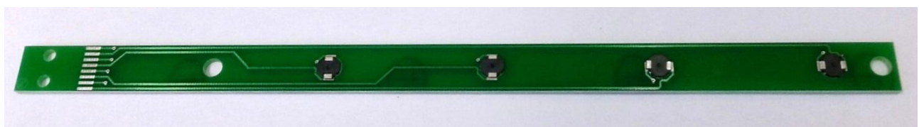
Fig. 7. In-house developed sampler: L \times W \times H = 300 \times 15 \times 3 \text{ mm} .
