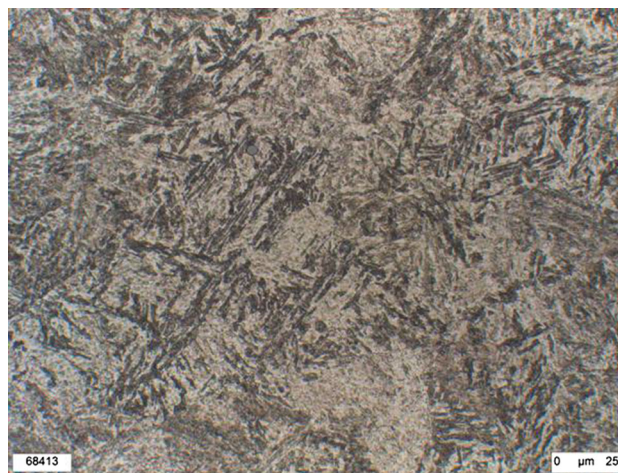
Fig. 1 Material microstructure after etching with Nital 5 %
