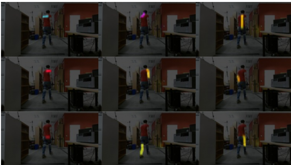
Figure 4.4: Sample body limb-maps generated by OpenPose [11] for an RGB images of SMAD.
