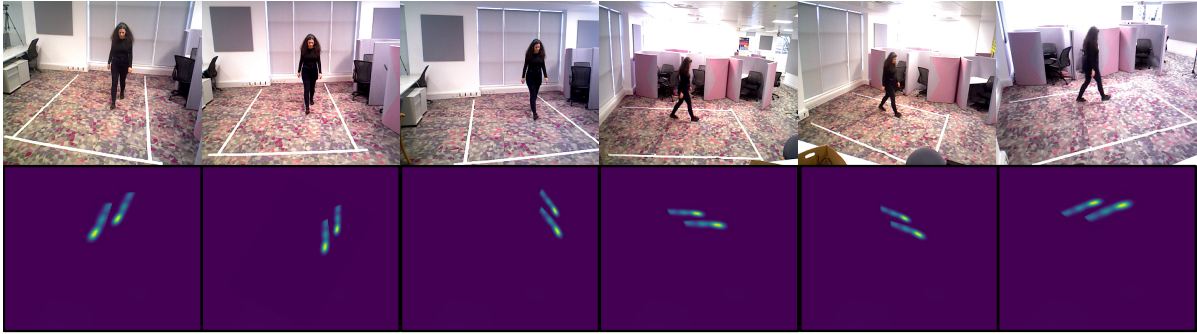
Figure 5.1: Sample images of a person walking in all six views, and the corresponding trajectory maps of her feet for each view.
