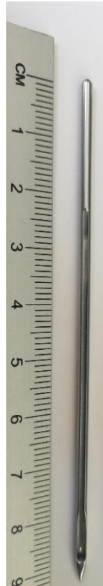
Figure 3-8 A Schmetz EP 11 Nm 230 tufting needle with a 1.0 mm diameter.
