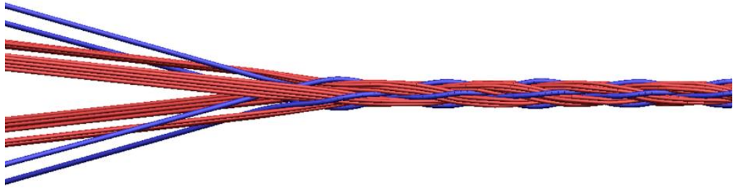
Figure 4-4 Simulated hybrid braid. Model yarns distinguished by material type and coloured according to direction travelled around the sinusoidal carrier path.
