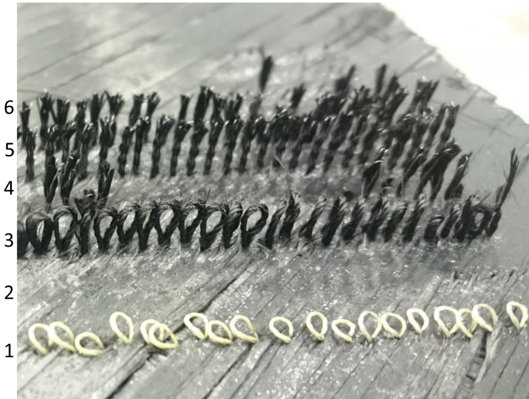
Figure 3-10 Underside of tufted panel, (1) Kevlar® yarn, (2) failed carbon fibre braid, (3) 4K carbon fibre thread, (4) titanium-carbon fibre 4 mm lay length hybrid braid, (5) titanium-carbon fibre 8 mm lay length hybrid braid, (6) titanium-carbon fibre 12 mm lay length braid.
