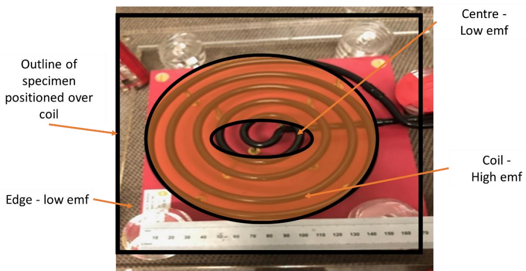
Figure 9-32 Schematic of coil position under test specimen with emf range and shape indicated.
