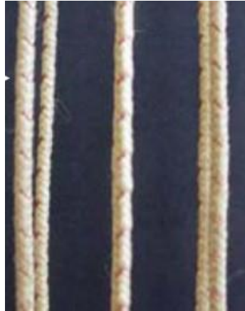
Figure 2-33 Kevlar® braided with copper wire [213].
