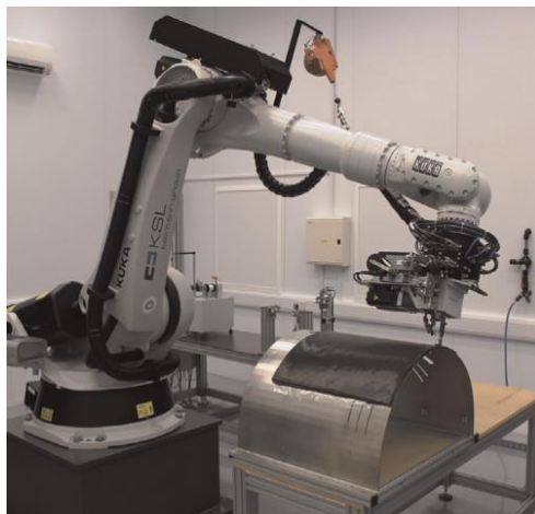
Figure 2-6 Robotic arm interfaced to KSL RS522 tufting head while tufting a simple single curvature preform on solid support backing [36].
