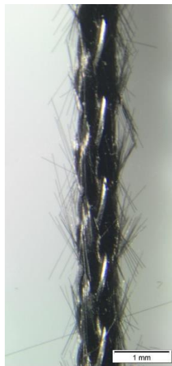
Figure 3-5 Titanium-carbon fibre hybrid micro-braid – 4 mm lay length.
