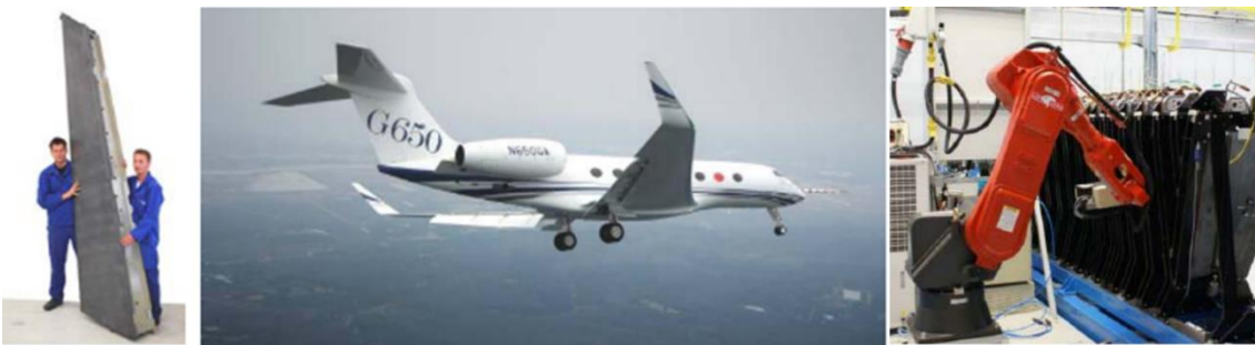
Figure 9-23 (Left) Induction welded G650 rudder torsion box. (Centre) First flight of G650 prototype aircraft. (Right) Induction weld robot and weld jig [275].
