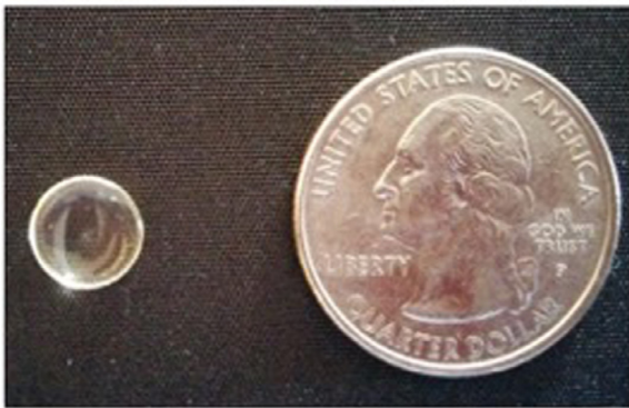
Fig. 4 – Image of 3D printed Ridley lens: the 3D printed lens shows good transparency but some notable surface roughness with irregularities. Permission granted from Fig. 1 of 14 .
