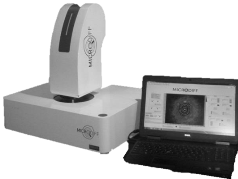
Figure 2 Photograph of the integrated MICRODIFF instrument for fast identification of clinical pathogens using elastic light scattering. Dimensions: 63x21x21 cm 3 , 10kg.
