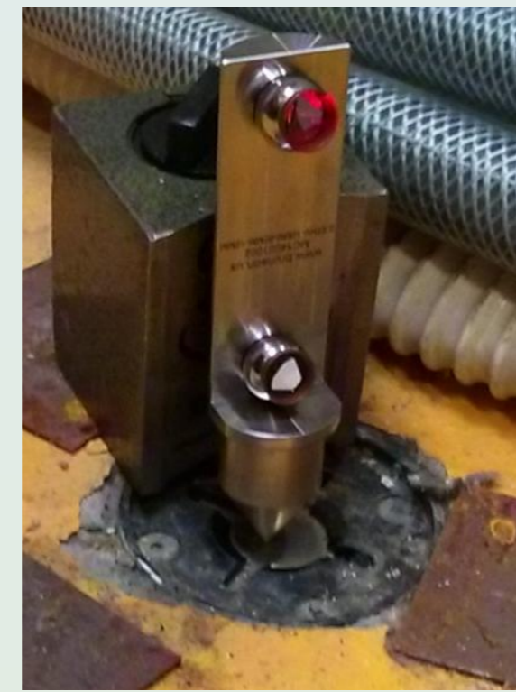
Measuring engraved cross mark
