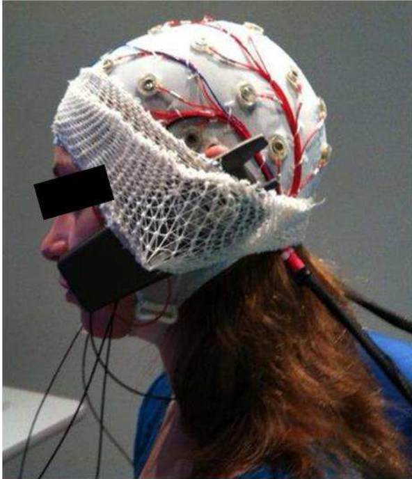
Fig 1. Position of MP during exposure period. Two optical temperature probes were positioned on the exposed cheek (left side) and on the control cheek (right side).
