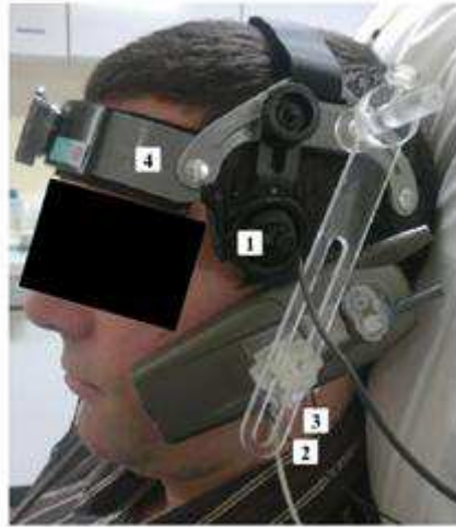
FIG. 2. Position of probes and MP during experimental sessions. The mobile phone and the 2 Mhz-probe (1) for transcranial Doppler sonography (TCD) were attached to the Doppler probe helmet (4). Two optical temperature probes were positioned on the left cheek (2) and under the left earlobe (3) (exposed side). A second TCD probe similar to the first and two optical temperature probes were also positioned on the right side (control side) for simultaneous symmetrical recording.
