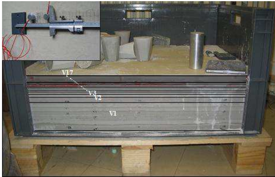
Figure 5: Superimposed layers of the test bed and measurement device on the surface.
