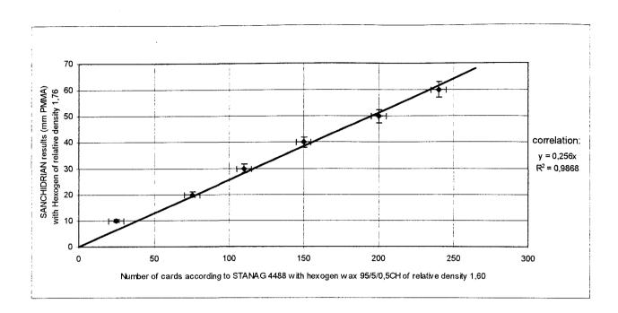
It can be seen that practically the same curve is obtained in both cases (see the coefficients of the equations of the lines given on the curves). It can be concluded from these correlations that there is equivalence between the two methods, and the following correspondence can be deduced:
