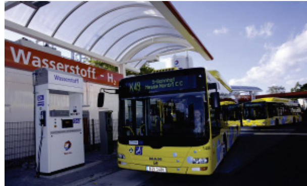
One of 14 hydrogen ICE Buses at the refueling station in Berlin
