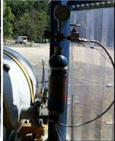
Figure 1 : sketch (dimensions in mm) and views of the 1 m 3 vessel (injection device of the fuel on the right picture)
