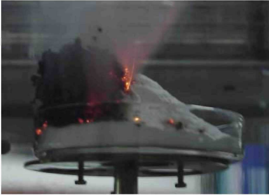
Figure 4: Smoke Powder 1 burning in the Tewarson apparatus operated by INERIS
