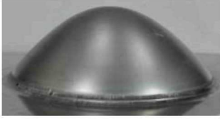
Photo 2: Bulged Plate (AL5754, Detonation, Pi=1.1 bar, Rounded Edge)
