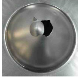
Photo 3: Cap Ejected (Al5754, Detonation, Pi=1.2 bar, Rounded Edge)
