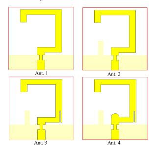
FIGURE 2. The design procedure of the proposed antenna.
