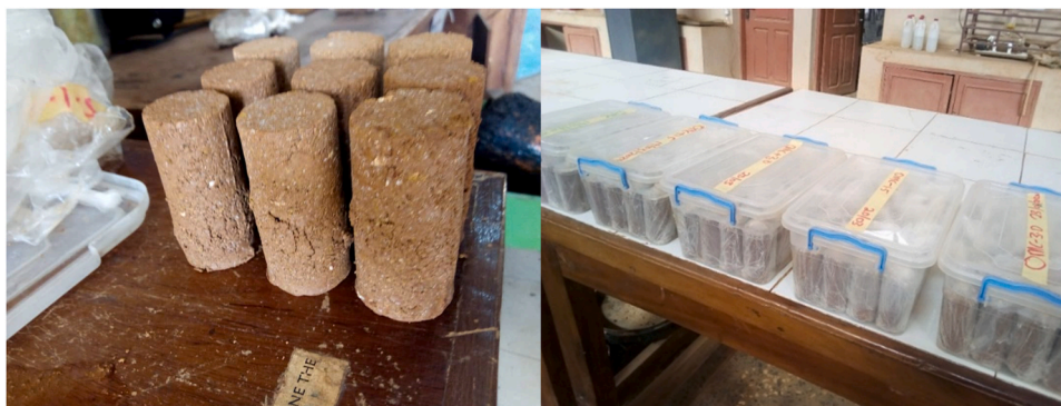
Fig. 10. Preparation and curing of UCS samples.
