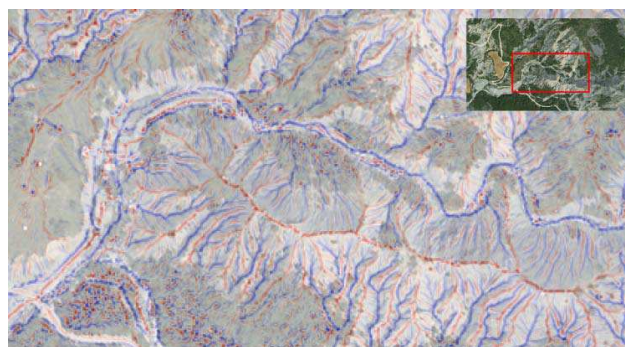
Fig. 5. CI computed on lidar data superimposed to the orthoimage.
