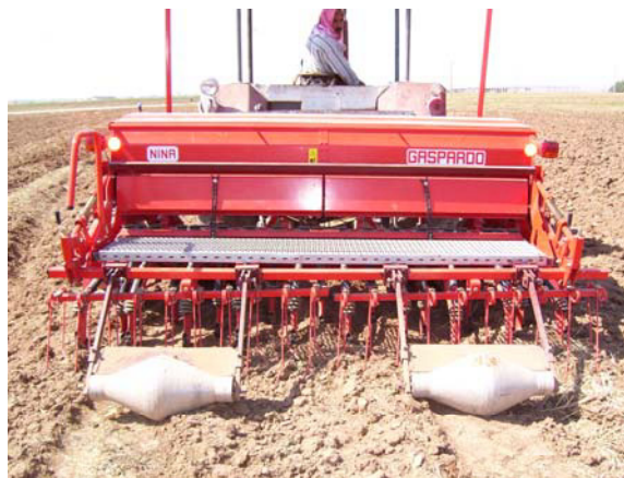
Figure 11. Rollers applied behind the seeder machine
