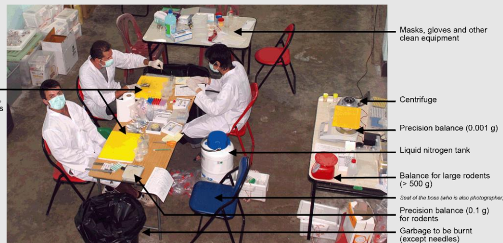
Figure 25: Example of organization of the field laboratory (CERoPath project, Nan province, 06/2008) (Photo: Morand S.)
