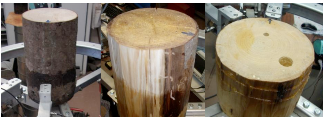
Figure 2. Tomography tests on the first log (from left to right: bark, debarked and drilled with two holes of diameter 1 cm and 2 cm).
