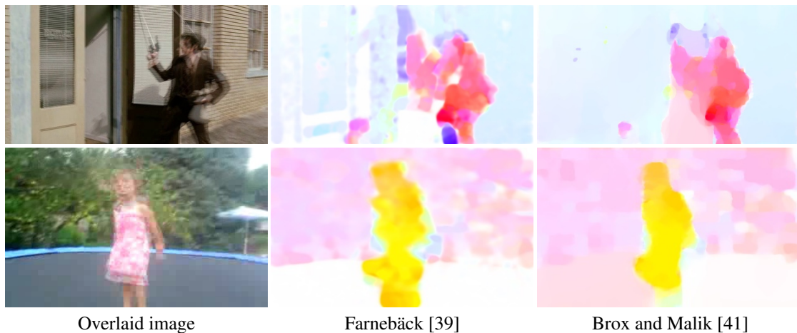
Figure 10: Examples from Hollywood2 (top) and YouTube (bottom). The left column shows the overlaid image of two consecutive frames. The middle and right columns are the visualization of two optical flow methods [39] and [41].
