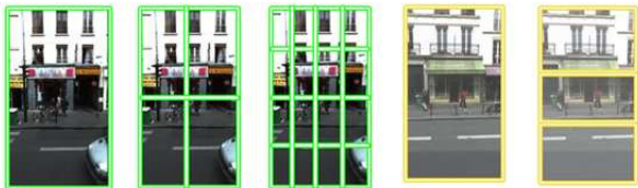
Figure 3. Taking into account spatial information in the image descriptor. Left: Illustration of the Spatial Pyramid Matching (SPM) scheme. Right: Illustration of the Street Context Slicing (SCS) technique.
