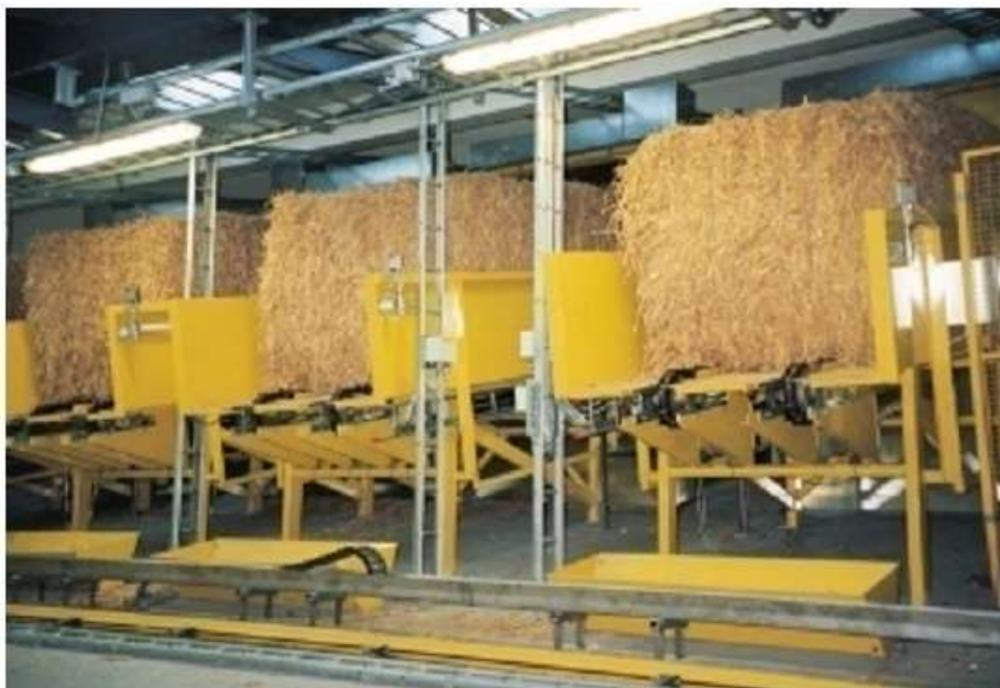
Figure 12. Straw bales in feeding line at Enstedværket Power Plant, Denmark
