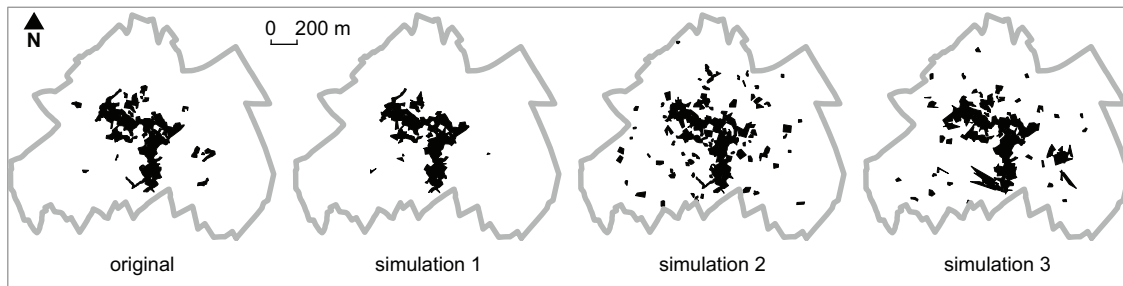
Figure 1: Original impervious polygons from the automatic dataset and three examples of impervious polygons simulations for the municipality of Jonquieres
